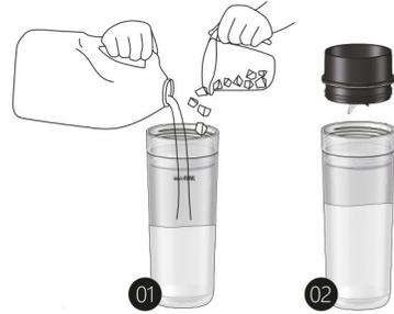
02. Attach the blade unit to the blender container.
